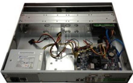
Figure 15-11 Connecting the HDD and the Power Cable
