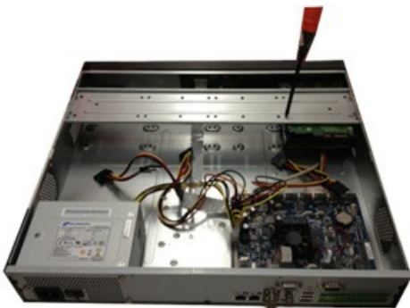
Figure 15-10 Placing the HDD
