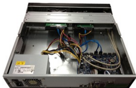
Figure 15-16 Connecting the HDD and the Power Cable
