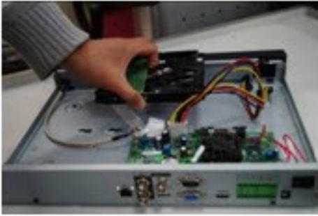
Figure 15-3 Placing the HDD
