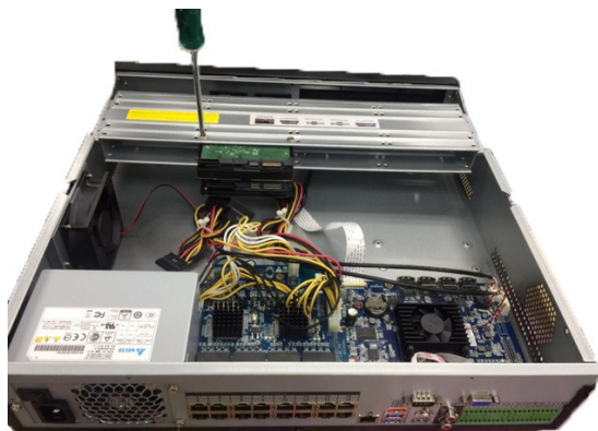
Figure 15-15 Placing the HDD
