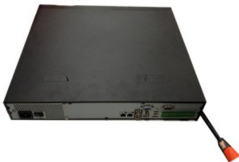
Figure 15-8 Removing the NVR Cover
