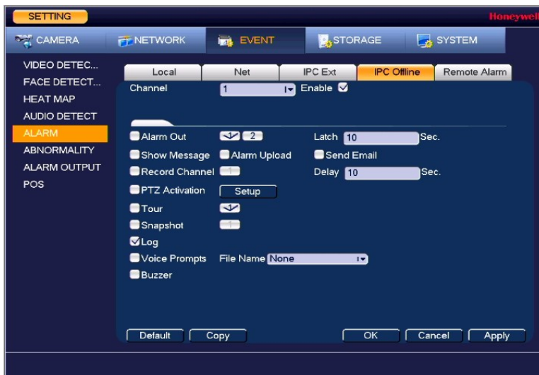
Figure 8-15 IPC Offline Alarm Configuration Tab
