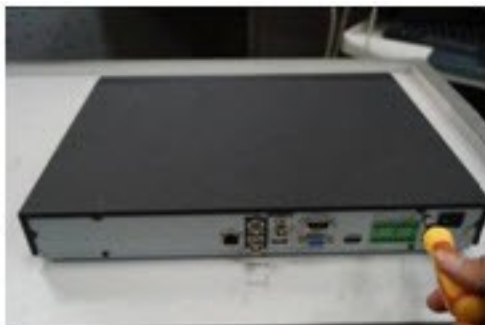
Figure 15-7 Securing the NVR Cover
