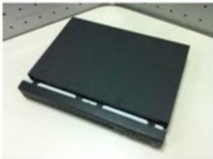
Figure 15-6 Replacing the NVR Cover
