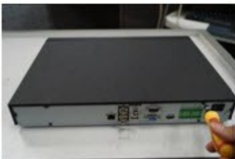
Figure 15-1 Removing the NVR Cover
