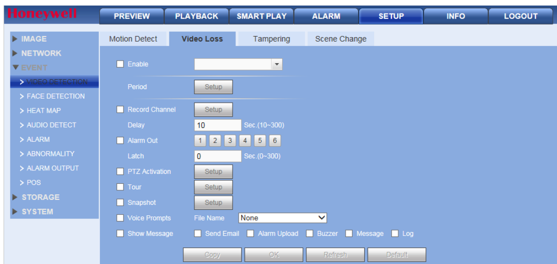
Figure 12-62 Video Loss Configuration Interface
