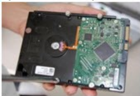
Figure 15-14 Loosening the Four Screws in the HDD Housing
