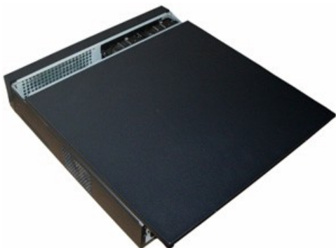
Figure 15-12 Replacing the NVR Cover
