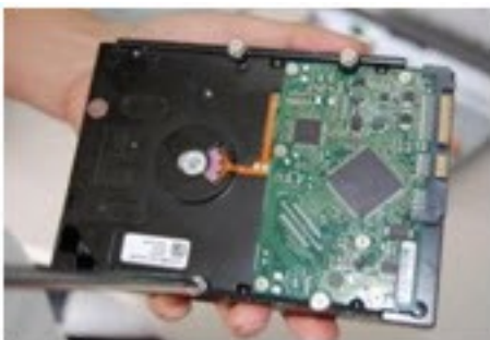
Figure 15-2 Loosening the Four Screws in the HDD Housing
