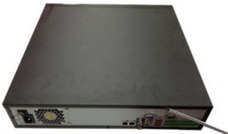
Figure 15-13 Removing the NVR Cover
